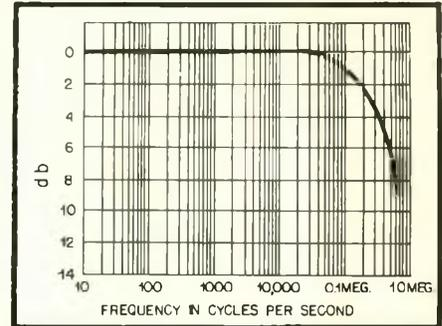
Fig. 2. Frequency response of this amplifier is flat at the low end and less than 3 db down at 200,000 cps, making it one of the widest-band designs in use today for audio.
