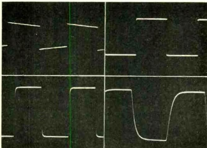
*Fig. 4.* These photos of oscilloscope traces show square-wave response at four frequencies—top row, left to right, 20 and 1000 cps; bottom row, 10,000 and 50,000 cps. Note the unusually short rise time even at 10,000 cps and the complete absence of evidences of instability despite a full 40 db of feedback. Effective output impedance is a fraction of an ohm, eliminating any tendency toward overshoot on transients.
