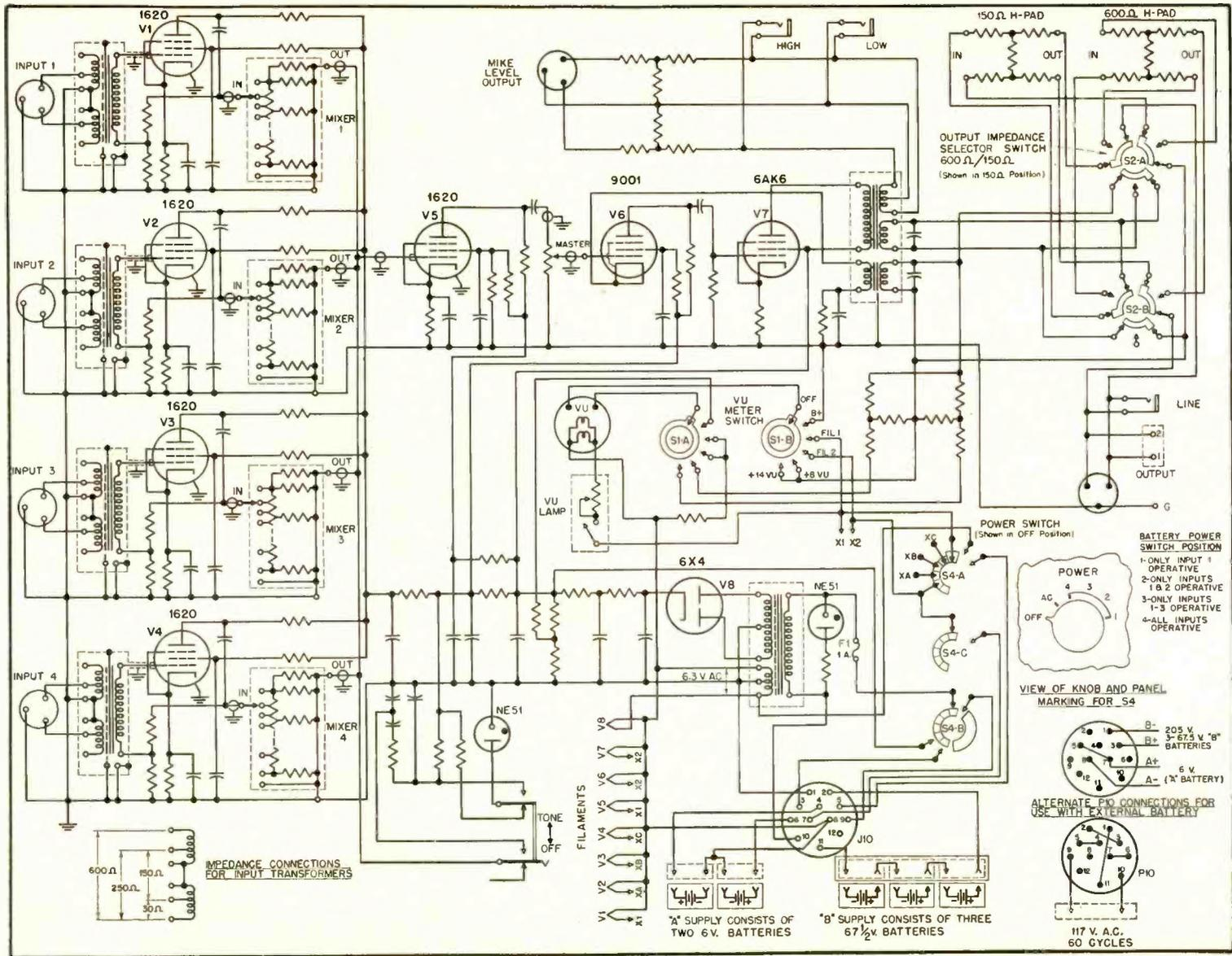
Fig. 3. Schematic of GE Type BA-6-A portable amplifier.
