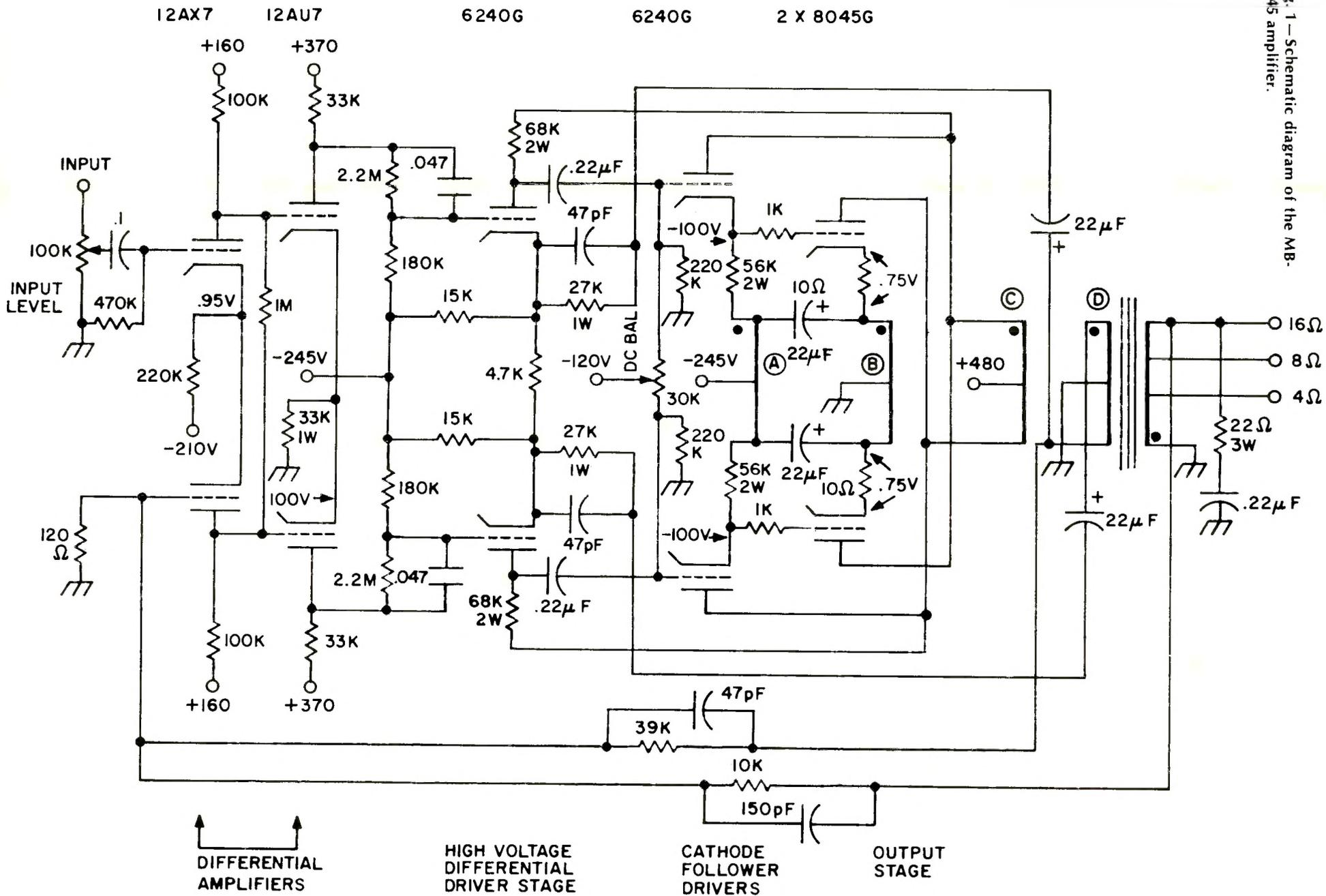
Fig. 1—Schematic diagram of the MB-3045 amplifier.
