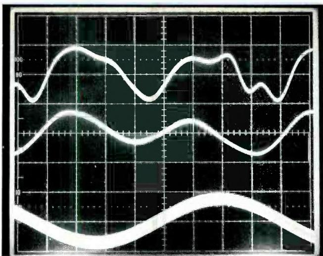
Fig. 4—MB-3045's SMPTM IM residual at 50 watts, Top; and 15.8 watts, Center; with input at bottom.
