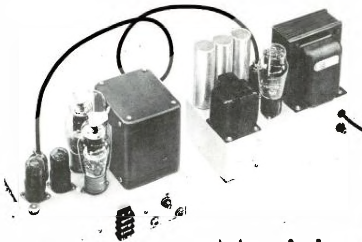
Fig. 1. The two chassis comprising the amplifier patterned after the "Williamson."
