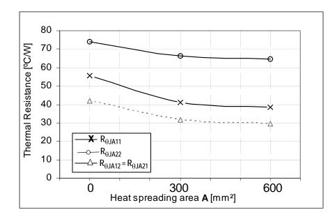
Figure 3. Device on Thermal Test Board  $R_{\theta J \textbf{A}}$
