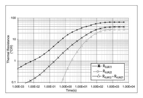
Figure 4. Transient Thermal Resistance  $R_{\theta JA}$  (1.0 W Step Response) Device on Thermal Test Board Area A = 600 (mm<sup>2</sup>)
