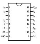
Figure 3. Pin Assignment for LCC
