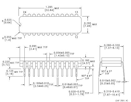
24 Lead Slim (0.300" wide) Ceramic Dual-in-Line Package (D) NS Package Number J24F
