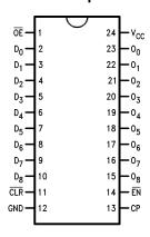
Figure 3. Pin Assignment for LCC
