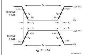
FIGURE 2. Test Input Signal Levels
