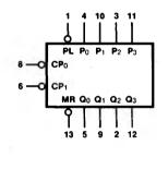
V<sub>CC</sub> = Pin 14 GND = Pin 7
