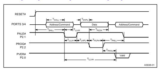
Figure 18. Slave Programming Mode in Word Dump or Data Verify Mode with Auto Increment
