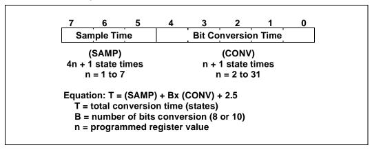
The converter is ratiometric, so absolute accuracy is dependent on the accuracy and stability of V<sub>REF</sub>. V<sub>REF</sub> must be close to V<sub>CC</sub> since it supplies both the resistor ladder and the analog portion of the converter and input port pins. There is also an AD\_TEST SFR that allows for conversion on ANGND and V<sub>REF</sub> as well as adjusting the zero offset. The absolute error listed is without doing any adjustments.
