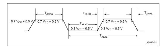
Figure 15. Input/Output Test Conditions
