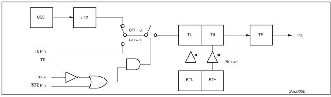
Figure 3. 83C749 Counter/Timer Block Diagram
