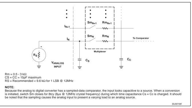
Figure 2. A/D Input: Equivalent Circuit
