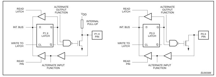
Figure 1. Port Bit Latches and I/O Buffers
