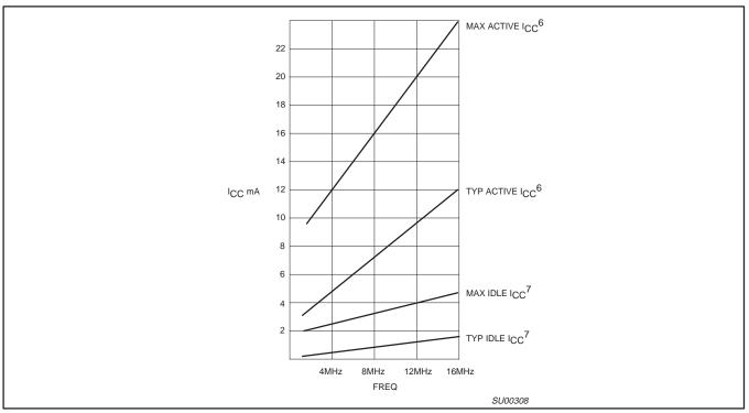
$\label{eq:state} \begin{array}{l} \mbox{Figure 6. } I_{CC} \mbox{ vs. FREQ} \\ \mbox{Maximum } I_{CC} \mbox{ values taken at } V_{CC} = 5.5 \mbox{V and worst case temperature.} \\ \mbox{Typical } I_{CC} \mbox{ values taken at } V_{CC} = 5.0 \mbox{V and } 25^{\circ} \mbox{C}. \\ \mbox{Notes 6 and 7 refer to AC Electrical Characteristics.} \end{array}$
