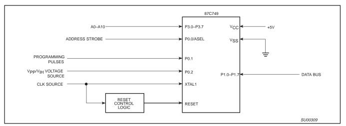
Figure 7. Programming Configuration
