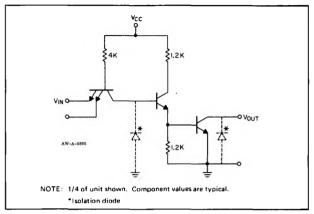
The 8881 is a Quad 2-Input NAND Gate with bare output collectors. Absence of an output pull-up structure allows the user complete freedom in the use of the 8881 in collector-logic (wired-AND) and similar applications. Proper pull-up resistor selection will allow as many as 50 outputs to be tied together.
