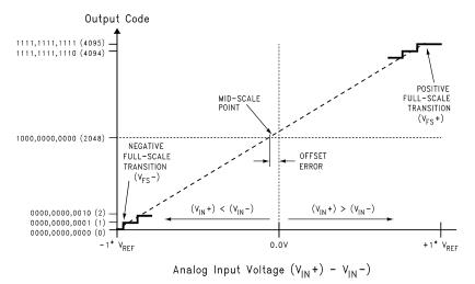
Figure 4. Transfer Characteristic
