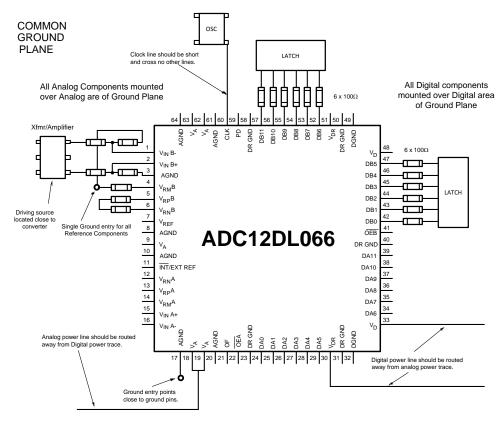
Figure 35. Example of a Suitable Layout
