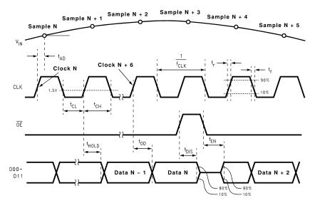
Figure 3. Output Timing
