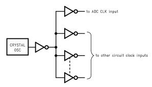
Figure 36. Isolating the ADC Clock from other Circuitry with a Clock Tree
