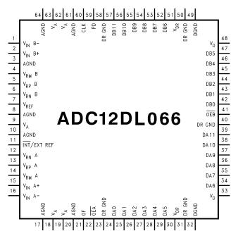
Figure 1. 64-Lead TQFP Package Package Number PAG
