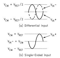
Figure 31. Expected Input Signal Range
