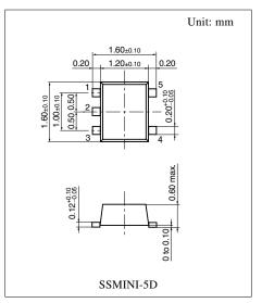
Note) The package of this product will be changed to lead-free type (SSMINI-5DA). See the new package dimensions section later of this datasheet.
