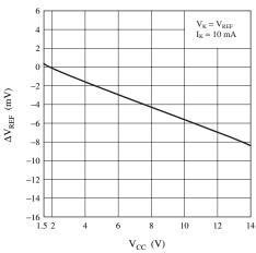
Reference voltage cathode current fluctuation
