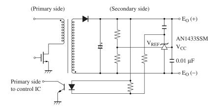
Note) As  $V_{CC}$  and cathode pin are separated,  $V_K$  can operate till 0.15  $V_{max}$  (at  $I_K = 10$  mA) at least.
