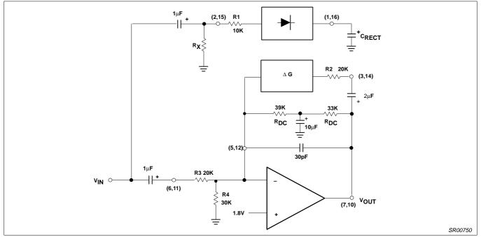
Figure 10. Automatic Level Control
