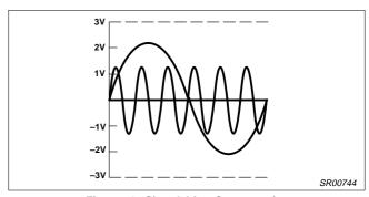
Figure 4. Signal After Compression
