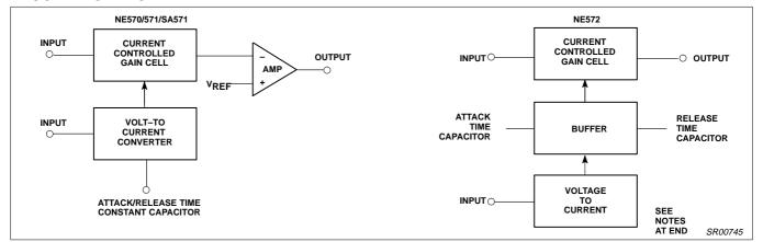
Figure 5. Block Diagrams
