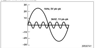
Figure 1. Original Signal Input
