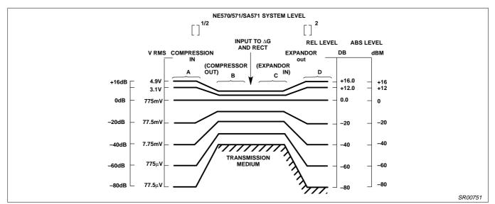
Figure 11. System Levels of a Complete Companding System
