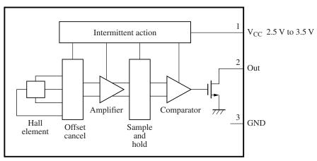
Note) The magnetism detection time should be longer than one intermittent action cycle ( $On = 200 \ \mu s$  and  $Off = 51 \ ms$ ).
