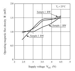
Operating magnetic flux density - Supply voltage
