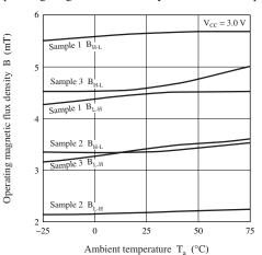
Operating magnetic flux density — Ambient temperature
