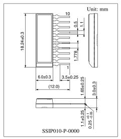
Note) The package of this product will be changed to lead-free type (SSIP010-P-0000A). See the new package dimensions section later of this datasheet.
