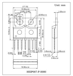
Note) The package of this product will be changed to leadfree type (HSIP007-P-0000B). See the new package dimensions section later of this datasheet.
