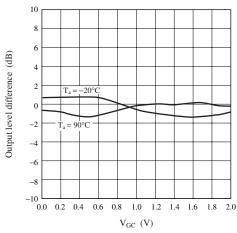
Output level — GC characteristic (Bi-phase — single phase output)
