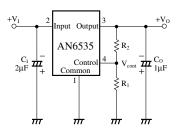
$$\begin{split} &V_{O} = V_{cont} \; \Big(\frac{R_{1} + R_{2}}{R_{1}}\Big) \\ &(V_{cont} \cong 3V, \, R_{1} = 3k\Omega) \end{split} \label{eq:Vo}$$
