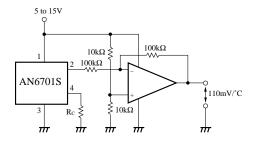
(c) When output polarity is inverted.
