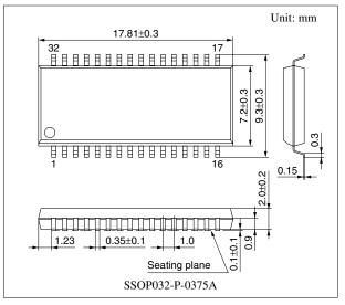
Note) The package of this product will be changed to lead-free type (SSOP032-P-0375C). See the new package dimensions section later of this datasheet.
