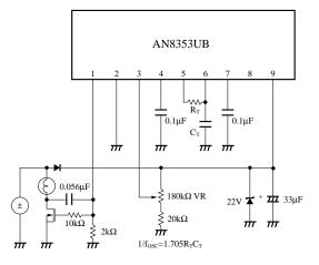
to generate pulses and input them to one end (Pin6) of the PWM comparator. The triangular wave frequency  $f_{\rm OSC}$  can be freely set from 50Hz to 10kHz, depending on the resistance value  $R_T$  connected between the square wave output Pin5 and triangular wave output Pin6, and capacity value  $C_T$  connected between the triangular wave output Pin6 and ground Pin2. The approximating expression for the then PWM frequency  $f_{\rm OSC}$  is ;
