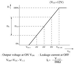
· Over voltage Detecting Voltage vs. Output
