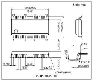
Note) The package of this product will be changed to lead-free type (HSOP030-P-0300A). See the new package dimensions section later of this datasheet.
