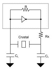
$C_L$  = 2\*( $C_P$  –  $C_S$ ), Where  $C_P$  = Load capacitance of crystal
