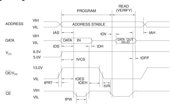
1. The Input Timing reference is 0.8V for  $V_{IL}$  and 2.0V for  $V_{IH}$ .
