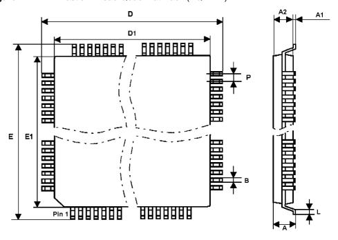
Table 9. 44-lead TQFP Package Dimensions (in mm)
