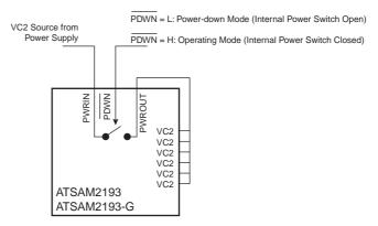
Note: High level for  $\overline{PDWN}$  is VC2 = 2.5V ±10%.
