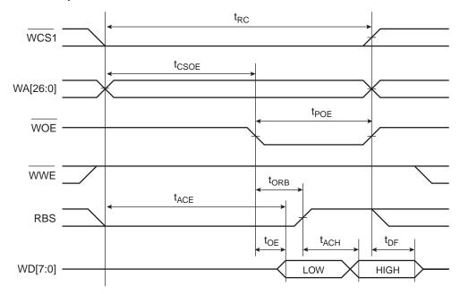
Figure 16. 8-bit SRAM Write Cycle
