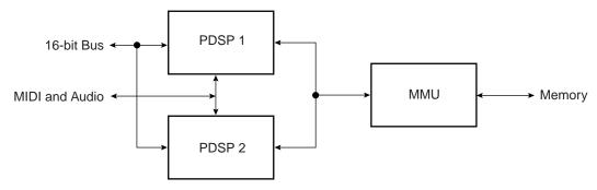
Figure 2. PDSP Block Diagram
