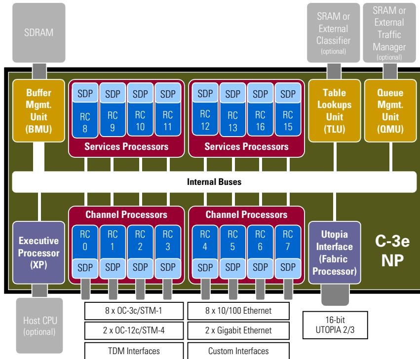
For aggregating even lower speed interfaces, the C-3e NP's Channel Processors can be connected to Motorola's TDM channel adapter products to provide highly cost-effective interface densities, without sacrificing functionality. For example, the TDM channel adapters will aggregate multiple T1/E1 lines consisting of multiple, independent, logical channels into a single C-3e NP Channel Processor.
