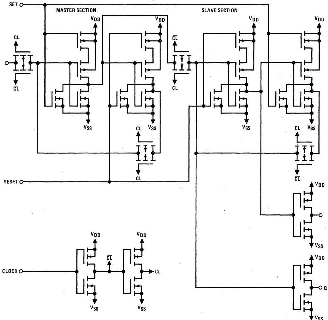
ALL P-SUBSTRATES ( ) CONNECTED TO V<sub>DD</sub>
