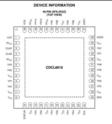
NOTE: Exposed thermal pad must be soldered to  $\mathrm{V}_{\mathrm{SS}}.$
