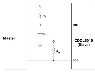
Figure 5. Serial Interface Connections
