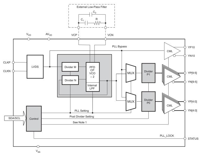
(1) Outputs can be disabled to floating. When outputs are left floating, internal 50 $\Omega$  termination to V<sub>DD</sub> pulls both YN and YP to V<sub>DD</sub>.
