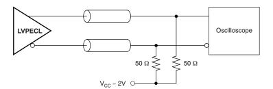
Figure 11. LVPECL DC Configuration During Device Test
