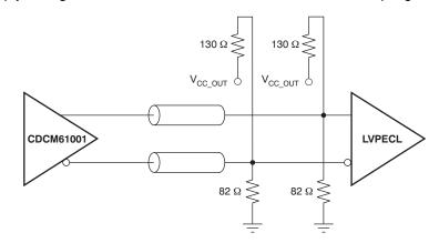
Figure 20. LVPECL Output DC Termination
