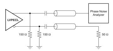
Figure 12. LVPECL AC Configuration During Device Test
