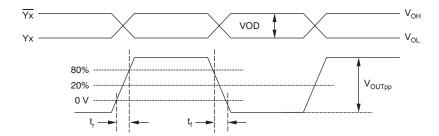
Figure 15. Output Voltage and Rise/Fall Times
