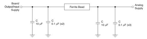
Figure 19. Recommended Power-Supply Decoupling
