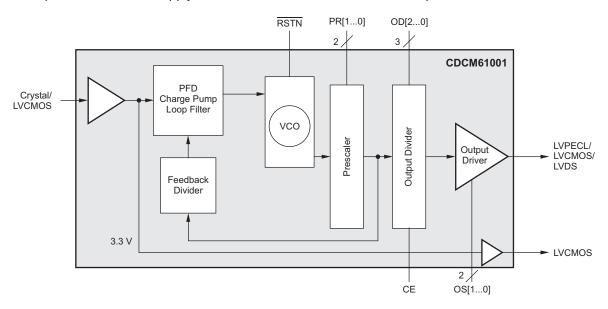
Figure 1. CDCM61001 Block Diagram
