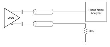
Figure 14. LVDS AC Configuration During Device Test
