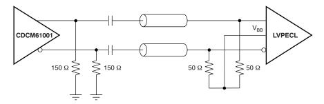
Figure 21. LVPECL Output AC Termination
