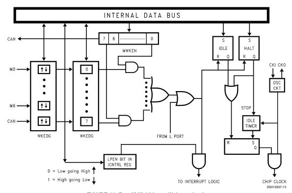
FIGURE 12. Port M Multi-Input Wake-up Logic
