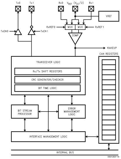
FIGURE 14. CAN Interface Block Diagram
