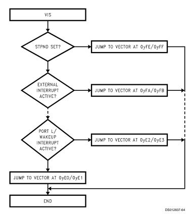
FIGURE 33. VIS Flowchart
