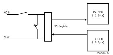
FIGURE 37. Loop Back Mode Block Diagram
