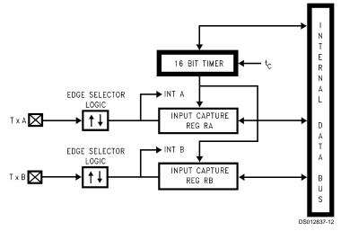
FIGURE 11. Timer in Input Capture Mode
