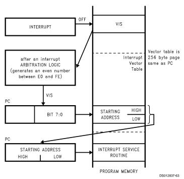
FIGURE 32. VIS Operation
