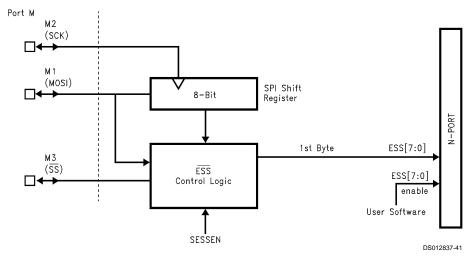
FIGURE 39. Programming the SPI Expander
