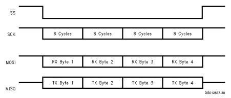
FIGURE 36. SPI Transmission Example
