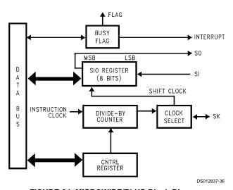
FIGURE 34. MICROWIRE/PLUS Block Diagram
