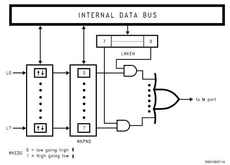
FIGURE 13. Port L Multi-Input Wake-Up Logic
