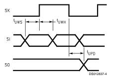
FIGURE 3. MICROWIRE/PLUS Timing Diagram
