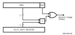
FIGURE 17. Acceptance Filter Block-Diagram
