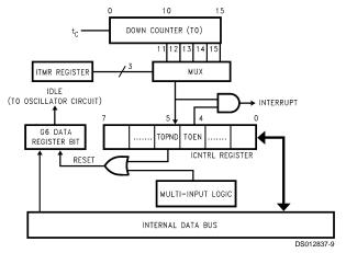
FIGURE 8. Functional Block Diagram for Idle Timer T0
