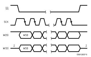
FIGURE 4. SPI Timing Diagram
