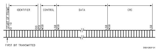
FIGURE 26. Order of Bit Transmission within a CAN Frame
