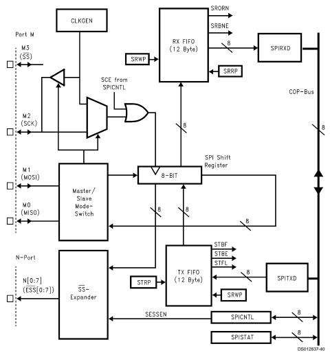
FIGURE 38. SPI Block Diagram
