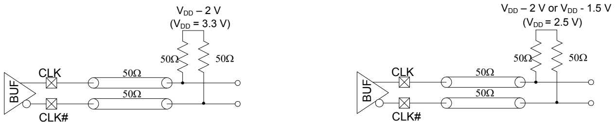
Figure 9. LVPECL Termination
