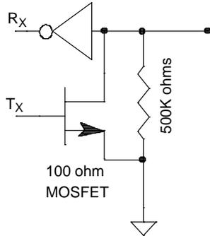
**BUS MASTER OPEN DRAIN CIRCUIT**
