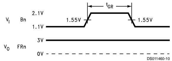
FIGURE 6. Receiver:  $t_{GR}$ , FRn(min) = 2V
