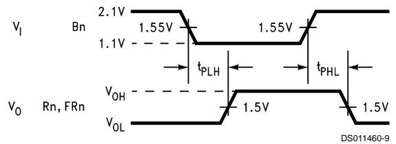
FIGURE 5. Receiver: Bn to FRn, Bn to Rn
