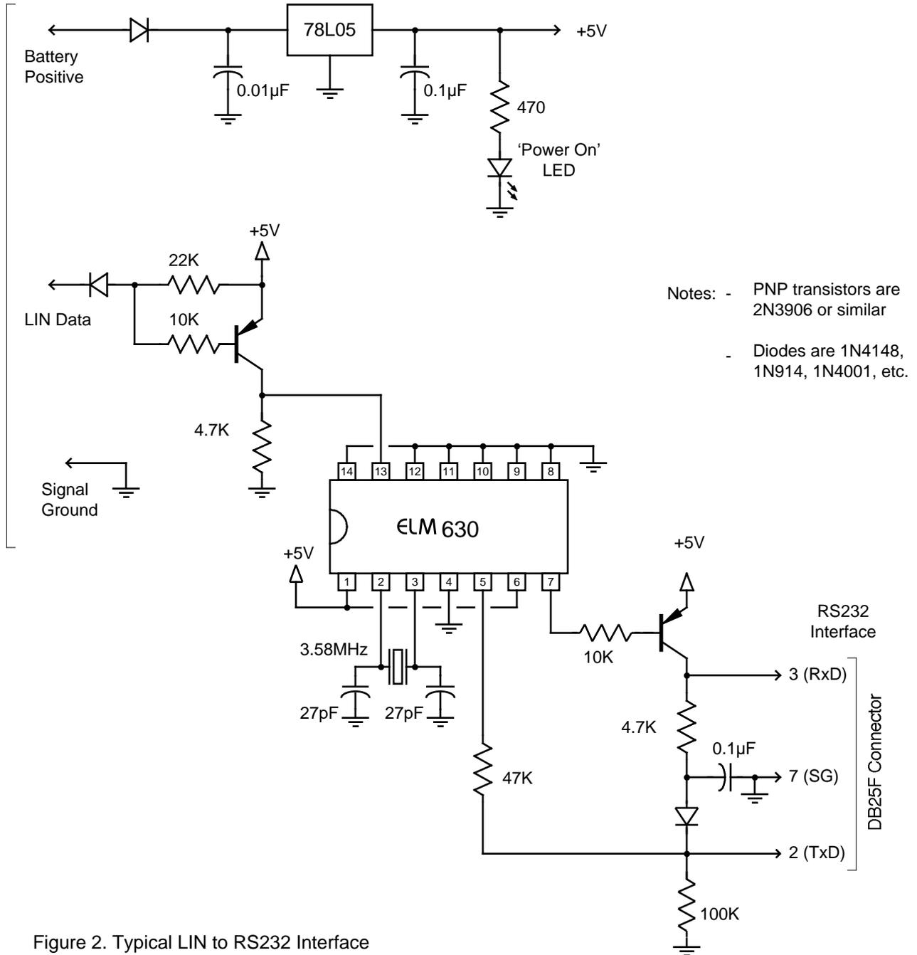
Figure 2. Typical LIN to RS232 Interface
