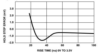
FIGURE 3. HOLD STEP ERROR vs S/H CONTROL RISE TIME
