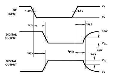
FIGURE 2. THREE-STATE TIMING CIRCUIT
