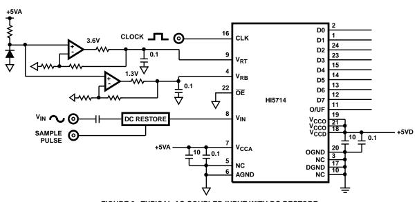
FIGURE 9. TYPICAL AC COUPLED INPUT WITH DC RESTORE
