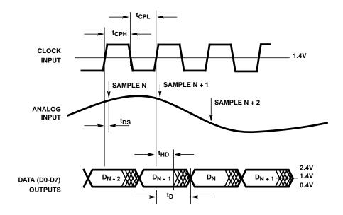
FIGURE 1. INPUT-TO-OUTPUT TIMING
