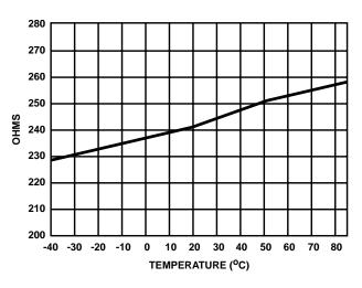
FIGURE 6. REFERENCE RESISTANCE vs TEMPERATURE
