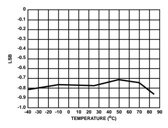
FIGURE 4. INTEGRAL LINEARITY ERROR vs TEMPERATURE
