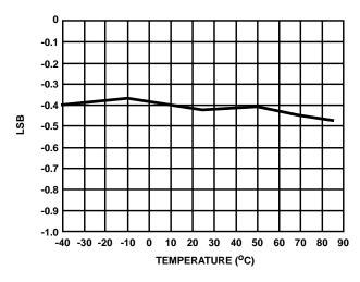
FIGURE 5. DIFFERENTIAL LINEARITY ERROR vs TEMPERATURE
