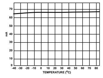
FIGURE 3. TOTAL  $I_{\mbox{CC}}$  vs TEMPERATURE
