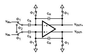
FIGURE 15. ANALOG INPUT SAMPLE-AND-HOLD
