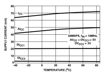
FIGURE 13. SUPPLY CURRENT vs TEMPERATURE
