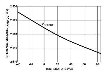
FIGURE 10. INTERNAL REFERENCE VOLTAGE ( $V_{\mbox{\scriptsize REFOUT}}$ ) vs TEMPERATURE
