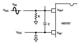
FIGURE 19. DC COUPLED SINGLE ENDED INPUT
