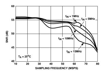
FIGURE 3. SNR vs SAMPLING FREQUENCY
