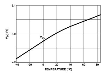
FIGURE 11. DC BIAS VOLTAGE (V<sub>DC</sub>) vs TEMPERATURE
