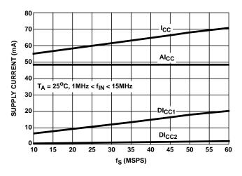
FIGURE 8. SUPPLY CURRENT vs SAMPLE CLOCK FREQUENCY
