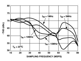
FIGURE 4. -THD vs SAMPLING FREQUENCY
