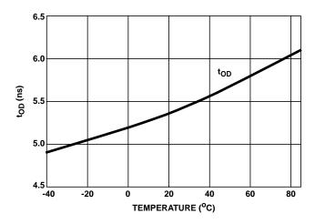
FIGURE 12. DATA OUTPUT DELAY ( $t_{\mbox{\scriptsize OD}}$ ) vs TEMPERATURE
