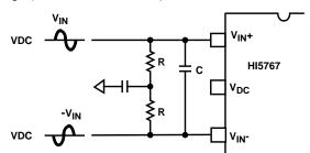
FIGURE 17. DC COUPLED DIFFERENTIAL INPUT
