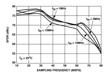
FIGURE 5. SFDR vs SAMPLING FREQUENCY
