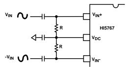
FIGURE 16. AC COUPLED DIFFERENTIAL INPUT
