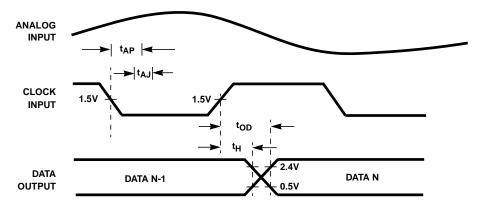
FIGURE 1. INPUT TO OUTPUT TIMING
