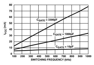
FIGURE 2. BIAS SUPPLY CURRENT vs FREQUENCY
