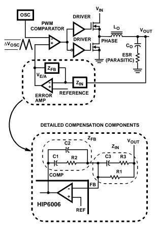
FIGURE 7. VOLTAGE - MODE BUCK CONVERTER COMPENSATION DESIGN
