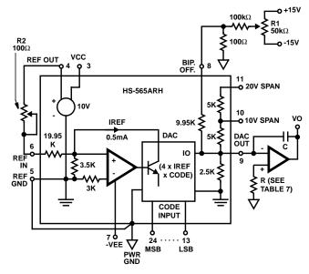
FIGURE 1. UNIPOLAR VOLTAGE OUTPUT
