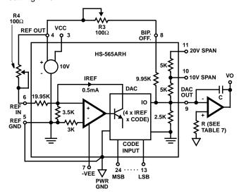
FIGURE 2. BIPOLAR VOLTAGE OUTPUT
