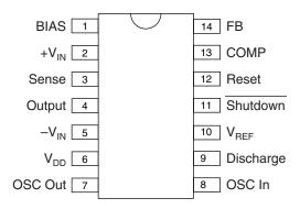
14 Pin SOIC/DIP Package
