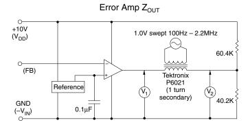
NOTE: Set Feedback Voltage so that  $V_{COMP} = V_{DIVIDE} \pm 1 mV$  before connecting transformer
