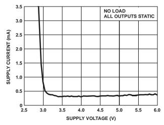
FIGURE 22. SUPPLY CURRENT vs SUPPLY VOLTAGE
