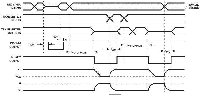
FIGURE 8. ENHANCED AUTOMATIC POWERDOWN, INVALID AND READY TIMING DIAGRAMS
