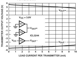
FIGURE 11. TRANSMITTER OUTPUT VOLTAGE vs LOAD
