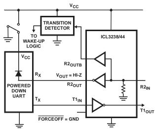
FIGURE 3. DISABLED RECEIVERS PREVENT POWER DRAIN
