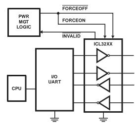
FIGURE 4. CONNECTIONS FOR MANUAL POWERDOWN
