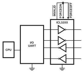
FIGURE 9. CONNECTIONS FOR AUTOMATIC POWERDOWN
