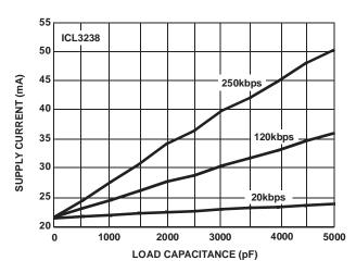
FIGURE 20. SUPPLY CURRENT vs LOAD CAPACITANCE WHEN TRANSMITTING DATA
