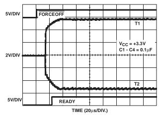
FIGURE 10. TRANSMITTER OUTPUTS WHEN EXITING POWERDOWN
