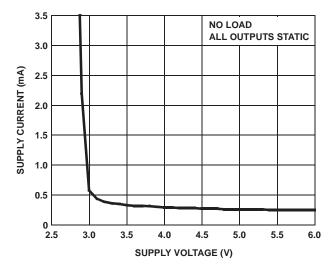
FIGURE 14. SUPPLY CURRENT vs SUPPLY VOLTAGE
