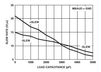
FIGURE 10. LOW SPEED SLEW RATE vs LOAD CAPACITANCE
