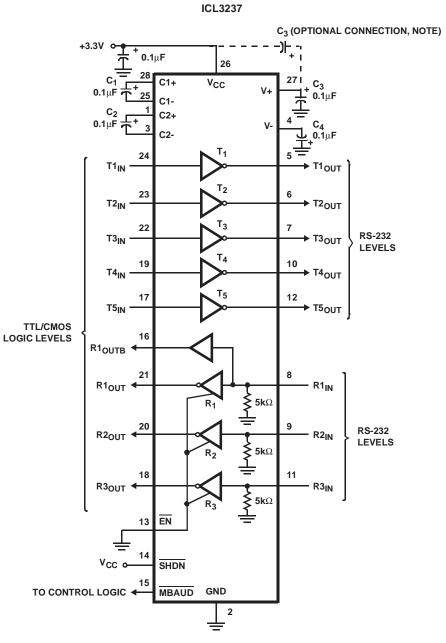
NOTE: THE NEGATIVE TERMINAL OF C<sub>3</sub> CAN BE CONNECTED TO EITHER V<sub>CC</sub> OR GND.
