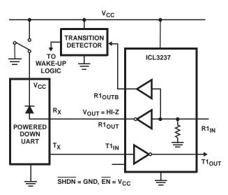
FIGURE 3. DISABLED RECEIVERS PREVENT POWER DRAIN
