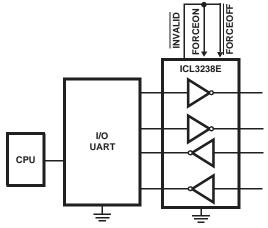
FIGURE 9. CONNECTIONS FOR AUTOMATIC POWERDOWN
