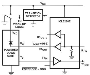
FIGURE 3. DISABLED RECEIVERS PREVENT POWER DRAIN
