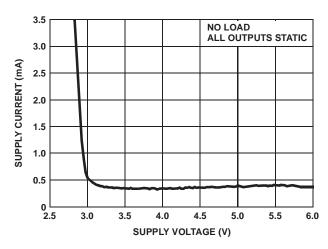
FIGURE 17. SUPPLY CURRENT vs SUPPLY VOLTAGE
