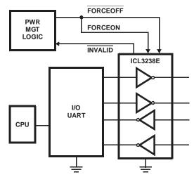
FIGURE 4. CONNECTIONS FOR MANUAL POWERDOWN
