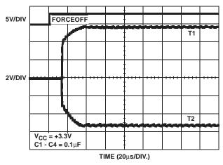
FIGURE 10. TRANSMITTER OUTPUTS WHEN EXITING POWERDOWN
