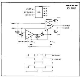
Figure 2. Maxim ICL7652 Block Diagram
