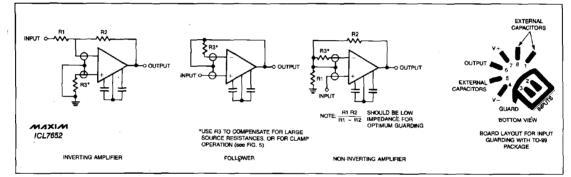
Figure 3. Input Guard Connection
