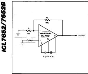
Figure 1. Maxim ICL:7652 Test Circuit
