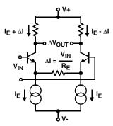
FIGURE 3. VOLTAGE TO CURRENT CONVERTER
