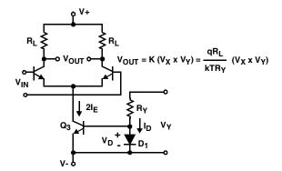
FIGURE 2. TRANSCONDUCTANCE MULTIPLIER
