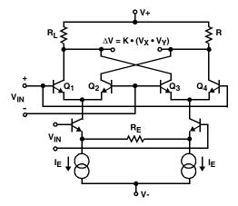
FIGURE 5. TYPICAL FOUR QUADRANT MULTIPLIER-MODULATOR
