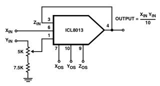
FIGURE 7B. MULTIPLIER CIRCUIT CONNECTION
