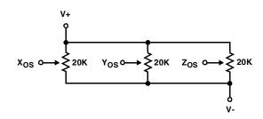
FIGURE 12. POTENTIOMETERS FOR TRIMMING OFFSET AND FEEDTHROUGH
