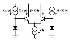
FIGURE 6A. CURRENT GAIN CELL
