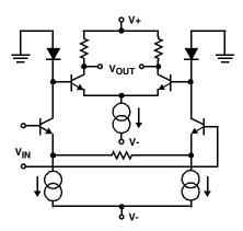
FIGURE 6B. VOLTAGE GAIN WITH SIGNAL COMPRESSION
