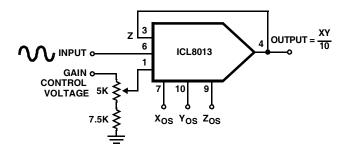
FIGURE 11. VARIABLE GAIN AMPLIFIER
