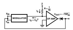
FIGURE 10A. SQUARE ROOT BLOCK DIAGRAM
